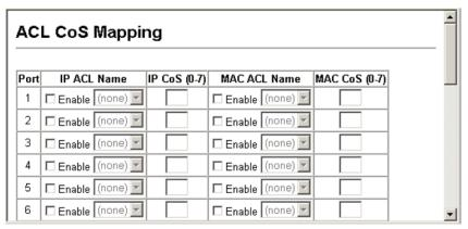
**CLI** – This example assigns a CoS value of zero to packets matching rules within the specified ACL on port 25.
