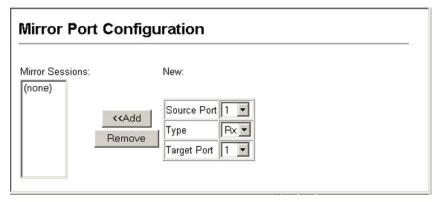
**CLI** – Use the interface command to select the monitor port, then use the port monitor command to specify the source port. Note that default mirroring under the CLI is for both received and transmitted packets.
