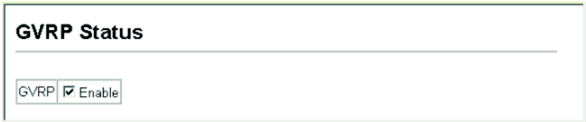
Figure 3-66 Globally Enabling GVRP
