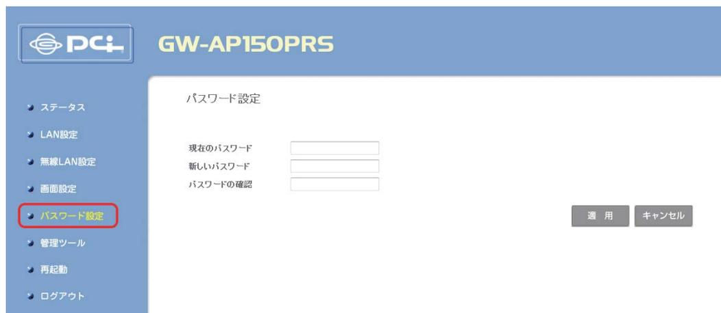
The screenshot shows the web management interface for the GW-API50PRS device. The title bar includes the PCi logo and the device name 'GW-API50PRS'. The left sidebar contains a menu with the following items: ステータス, LAN設定, 無線LAN設定, 画面設定, **パスワード設定** (highlighted with a red box), 管理ツール, 再起動, and ログアウト. The main content area is titled 'パスワード設定' and contains three input fields: '現在のパスワード', '新しいパスワード', and 'パスワードの確認'. Below the input fields are two buttons: '適用' and 'キャンセル'.
