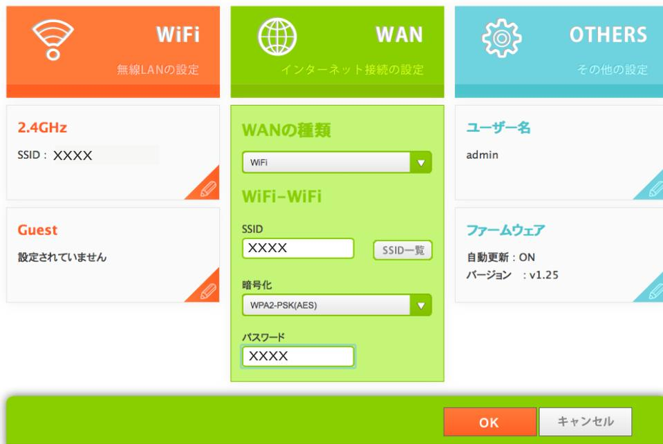
The screenshot shows the 'WAN' configuration screen after completion. The 'WiFi' tab is selected. Under 'WiFi-WiFi', the SSID is 'XXXX', the encryption is 'WPA2-PSK(AES)', and the password is 'XXXX'. The 'SSID一覧' button is visible. At the bottom, the 'OK' button is highlighted in red, and the 'キャンセル' button is visible.
