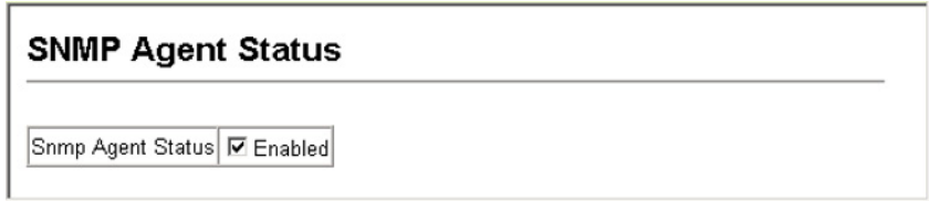
Figure 3-23 Enabling SNMP Agent Status
