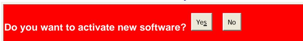
Press, “yes” then you get new code to execute, **however, after activate the new code**, better to press “**reset button**” at front panel so that the new default setting will be also updated, because different version code is sometimes with different initial default setting
